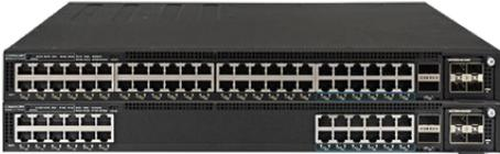
The RUCKUS ICX 7550 multigigabit models come in 24- and 48-port offering class leading multigigabit port density with a mix of 2.5G and 2.5/5/10G ports delivering the ultimate solution for Wi-Fi 6 access points Ethernet connectivity today while providing plenty of future proofing for deploying future generations of Wi-Fi APs.
